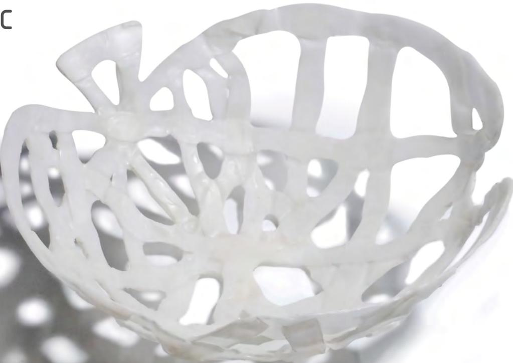
Bowl made of recycled HDPE (High-density polyethylene) bottles, and produced by a manual molding system which consists of controlled heating, taking advantage of the thermal properties of the material.
